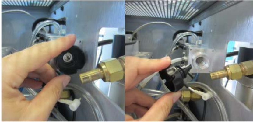
Picture 3: Unscrew the corona needle. The four cavities sideways at the needle can be used with a screw driver to unscrew the needle if it stuck. Take out the needle carefully without hitting walls with the needle tip.
