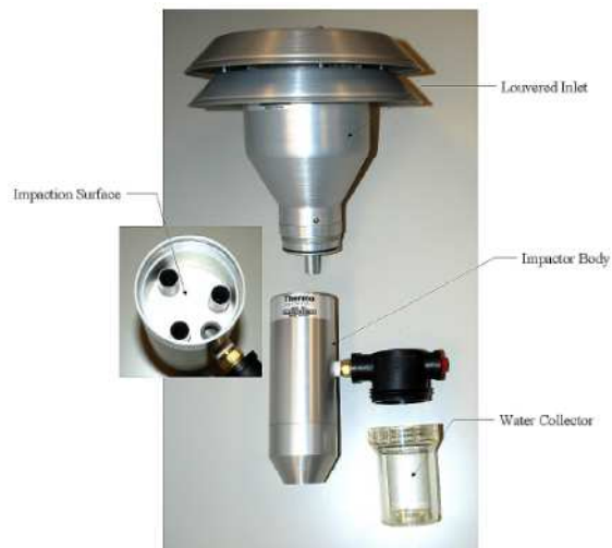
Figure 3-1 The Components of the PM 10 Inlet. The Impaction Surface is Located in the Bottom Part.
