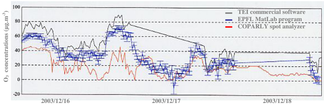
Graph 3 : O 3 concentrations calculated with EPFL and TEI programs, compared to analyzer results
